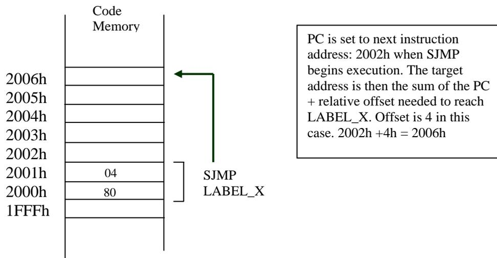
An advantage of relative addressing is that the program code is easy to relocate in memory in that the addressing is relative to the position in memory.
