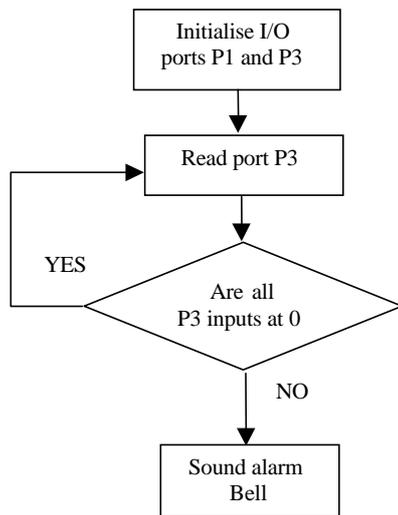
**Figure 2.2 ALARM\_1 Program flow chart**
