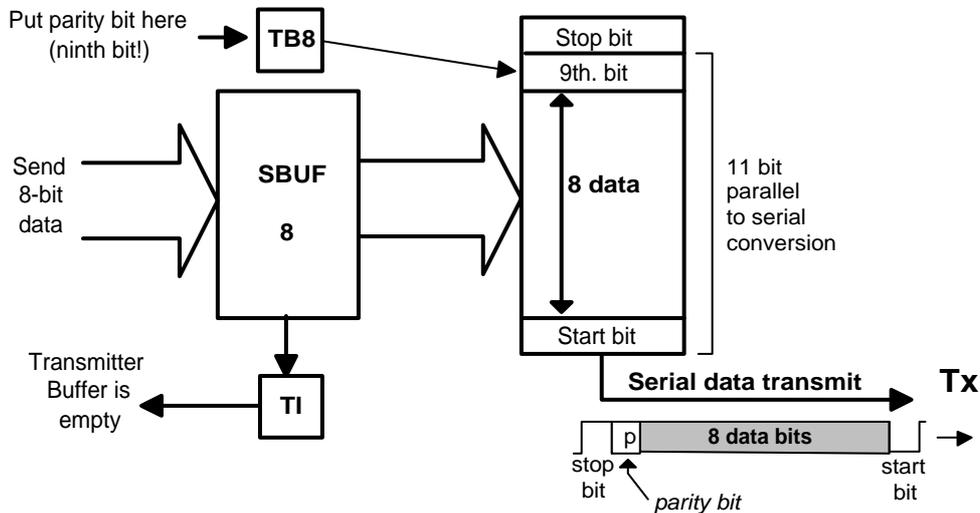
**Figure 6.5** Block diagram of UART transmitter, using the 9<sup>th</sup>. bit
