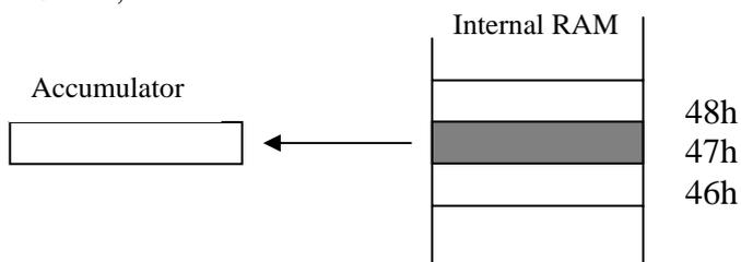
The instruction reads the data from Internal RAM address 47h and stores this in the accumulator. Direct addressing can be used to access Internal RAM , including the SFR registers.
