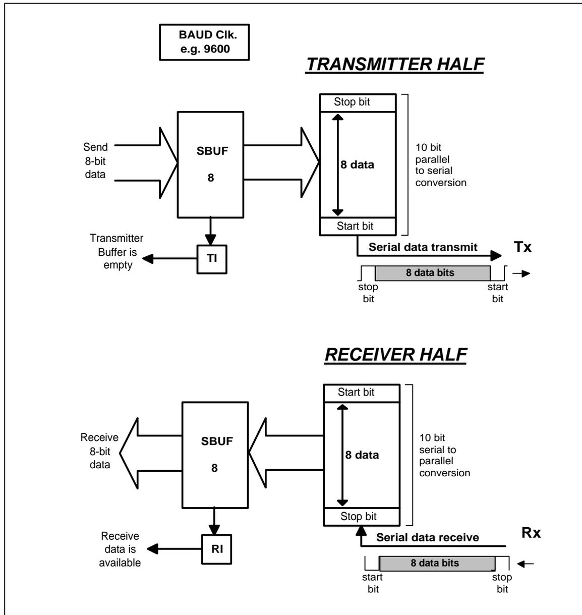
Figure 6.4 UART block diagram
