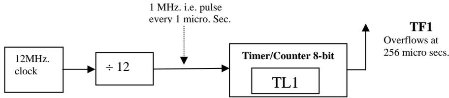
If the timer is initialised to zero it will count 256 microseconds before overflow. If the timer is initialised to a value of 252, for example, it will count just 4 microseconds before overflow. Thus this timer is programmable between 1 microsecond and 256 microseconds.
