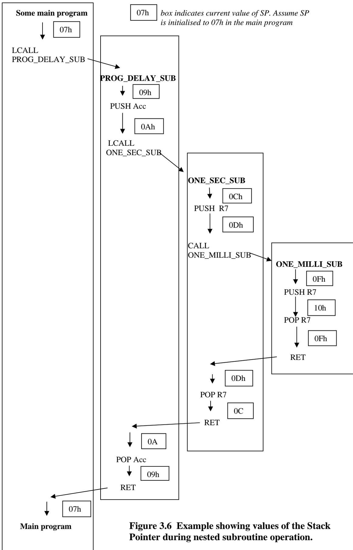
**Figure 3.6 Example showing values of the Stack Pointer during nested subroutine operation.**
