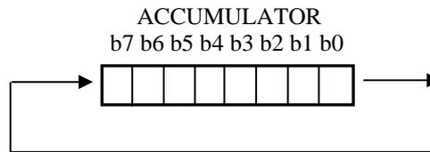
RRC A ; Rotates to the right and includes the carry bit as the 9<sup>th</sup> bit.
