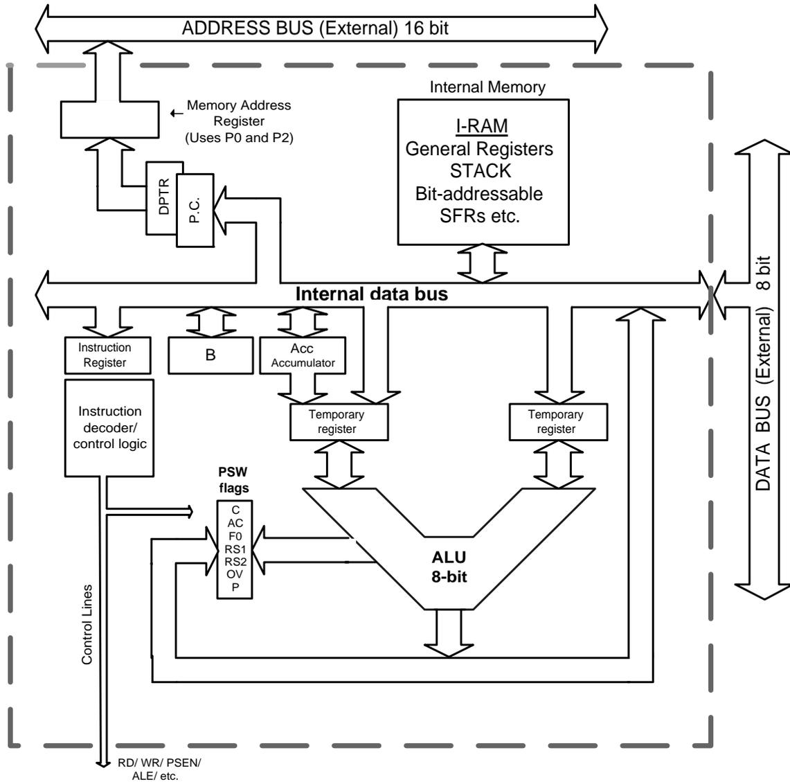
Figure 1.1 8051 functional block diagram.
