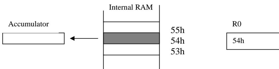
Note the @ symbol indicated that the indirect addressing mode is used. R0 contains a value, for example 54h, which is to be used as the address of the internal RAM
