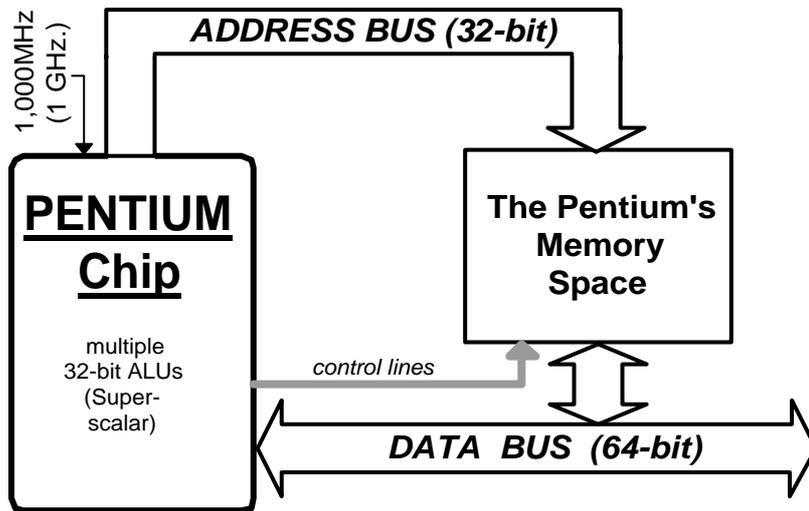
Figure 1.3 Simplified diagram of a Pentium processor
