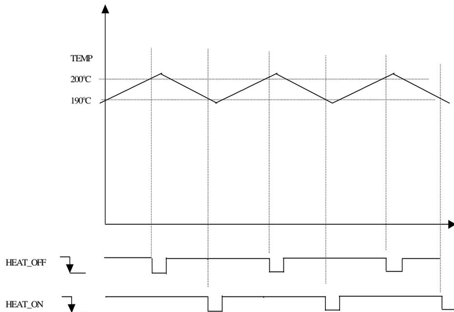
**Figure 4.3 Timing diagram for the oven control**
